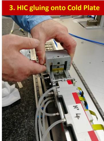
3. HIC gluing onto Cold Plate
