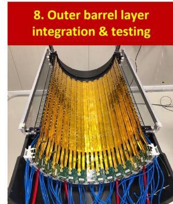
8. Outer barrel layer integration & testing
