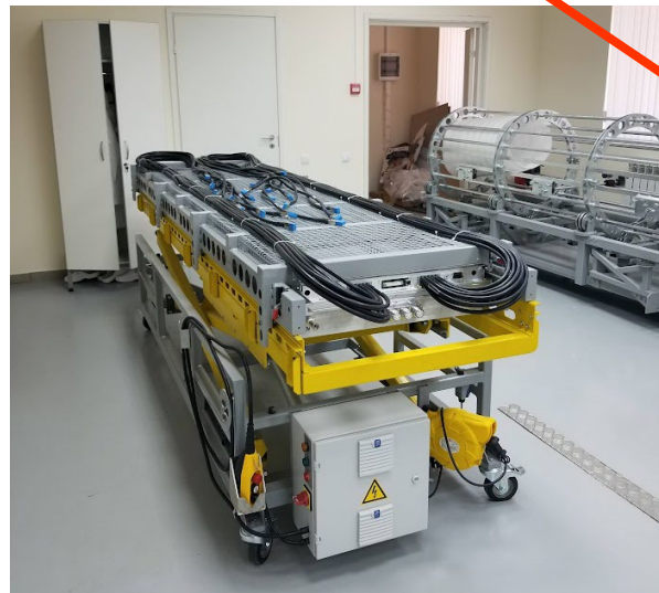
The TOF installation bench is fully assembled and tested in the VBLHEP
