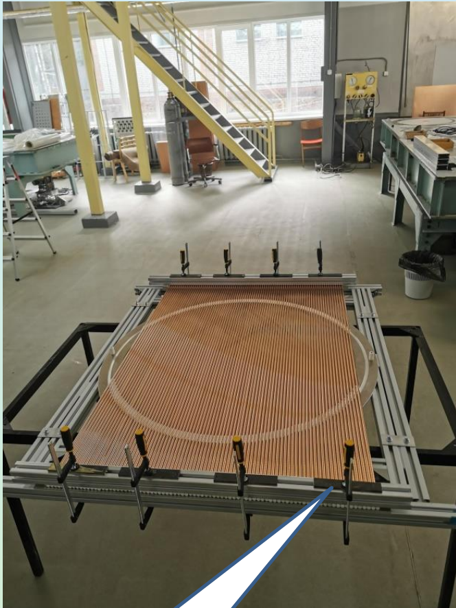
Frame for pre-tensioning of tubes
