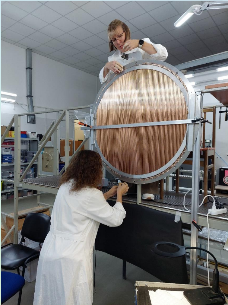
installation of anode wires
