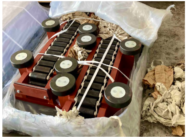
Requirement for the smooth motion of roller skates: \pm 0.5 mm
