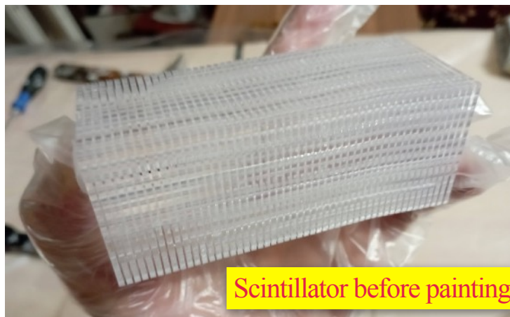
Final module assembly: 200 layers of 1.5 mm scintillator + 0.5 mm lead
