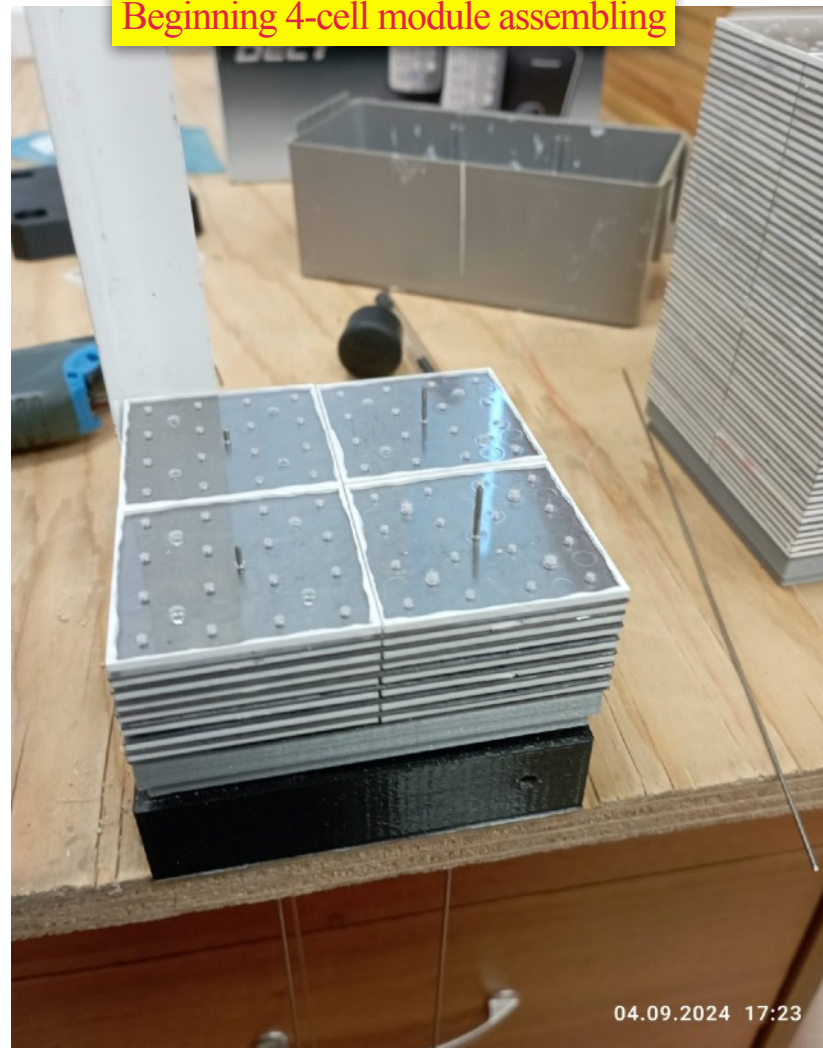
Final module assembly: 200 layers of 1.5 mm scintillator + 0.5 mm lead
