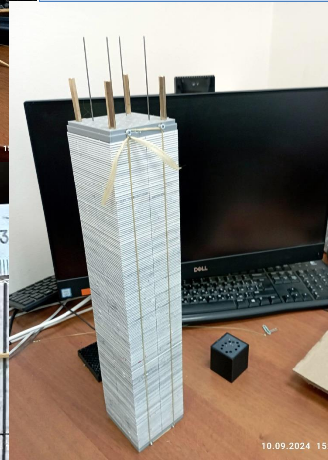
4-cells module assembled and tied with a Kevlar rope
