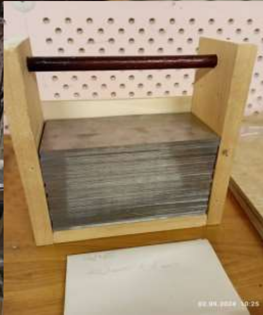
Box for 200 plates of 85x168 mm 2 – it is blanks for the press Has a weight ~20 kg
