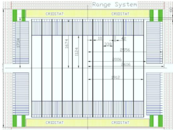
In total (basket walls + structural material): 20 mm of carbon fiber
