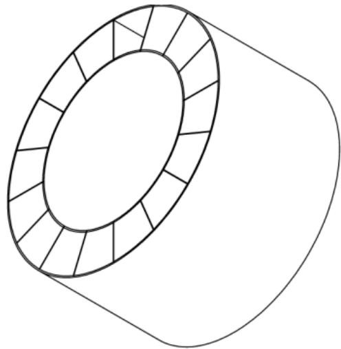
In total (basket walls + structural material): 24 mm of carbon fiber, 16 sectors
