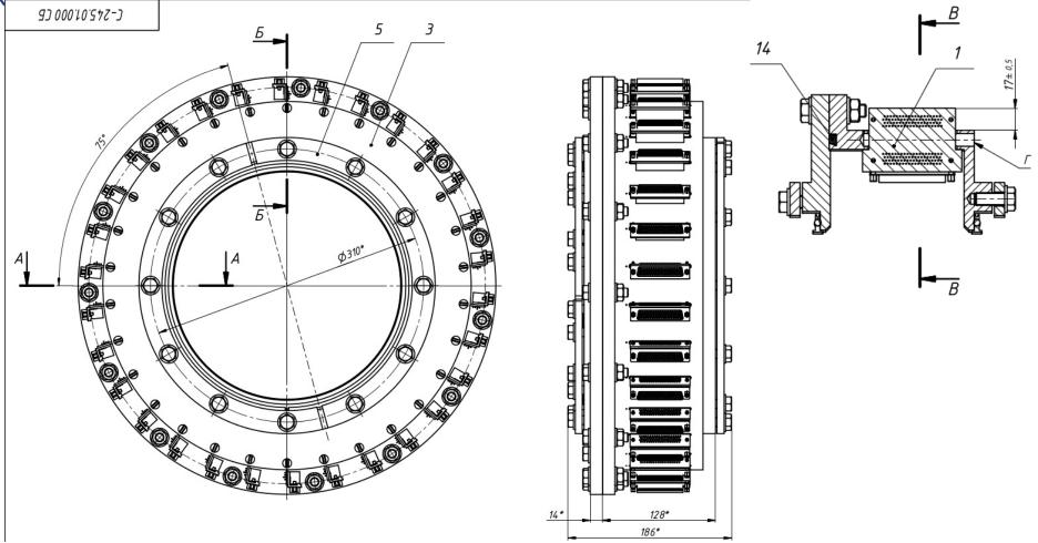
A barrel with 30 pcb boards with 78-pin connectors DHR-78F (DS1038-78F) will be installed on one side of the cryostat at large side flanges. The boards are already manufactured by REZONIT and received in JINR. Two barrels are ordered and expected to be received in JINR 28.12.2024.
