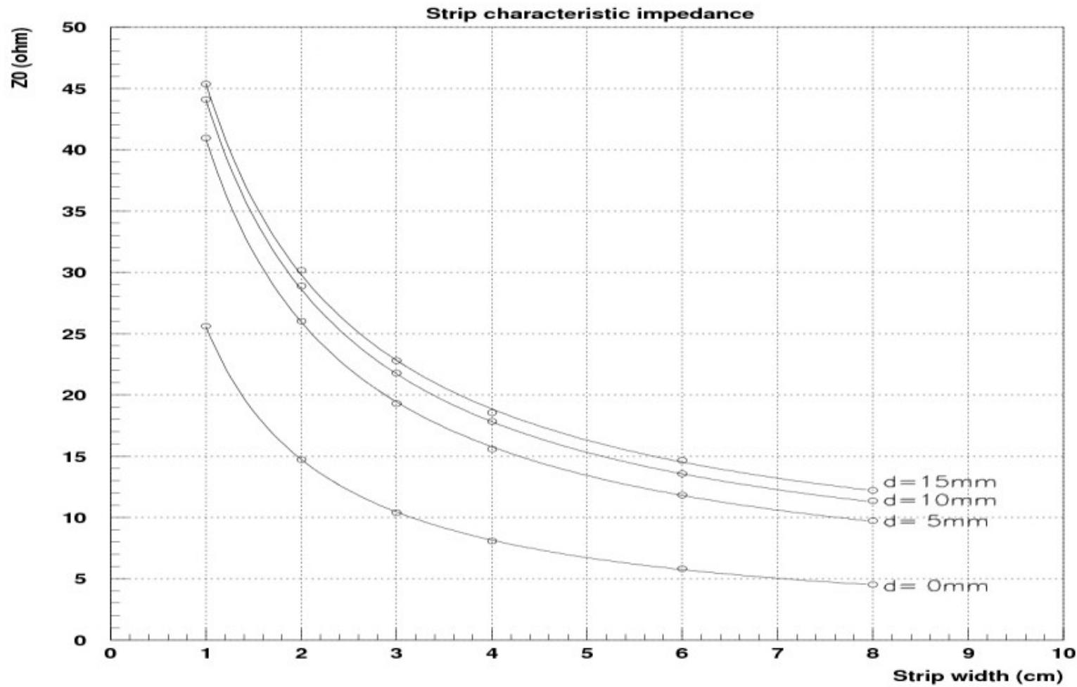
The dependence of the wave resistance of the strips on the width of the strips and the distances between the strip plane and the absorber plate,  $d = 0\div 15\text{ mm}$
