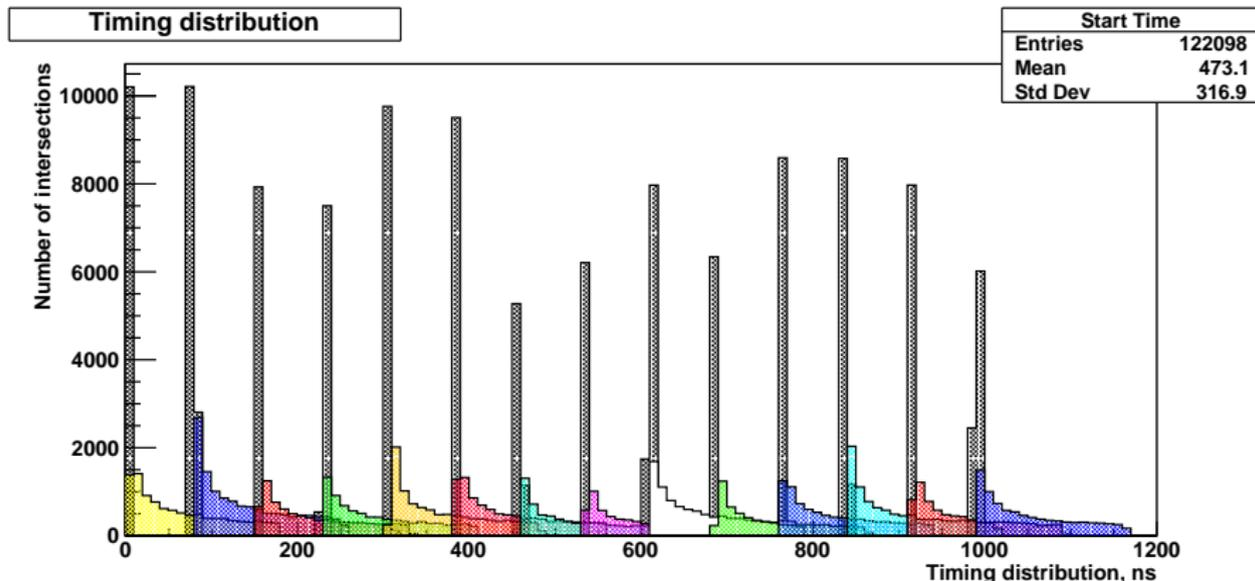
**Figure 3:** Timing distribution averaged by 100 time slices. Grey area – time of the intersection of the sensitive volume by the sample particle without taking into account the electron avalanche. Coloured area – ST response time distribution.
