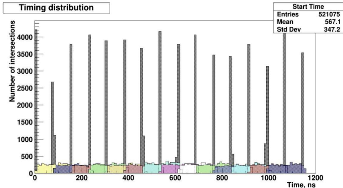
**Figure 6:** Timing distribution averaged by 400 time slices. Grey area – time of the intersection of the sensitive volume by the sample particle. without taking into account the electronic avalanche. Coloured area – ST response time distribution.
