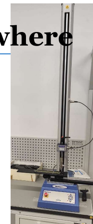
Peel test station
