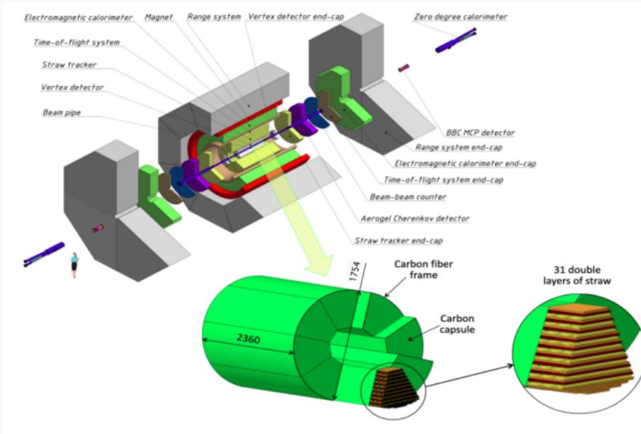
Straw diameter: 10mm thickness  $36\mu\text{m}$  PET
