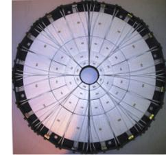
Hodoscopes of scintillator cells
