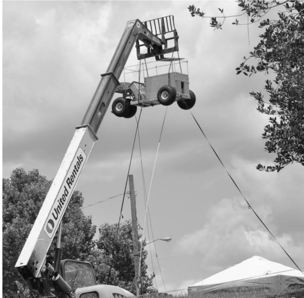
Fig. 4. Mobile inelastic neutron scattering system background measurements (up to 6.7 m above the ground).
