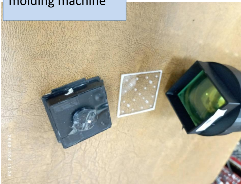
4 scintillators plates after injection molding machine
