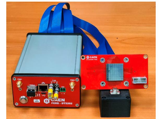
Pic. 18 – 8-tile telescope setup
