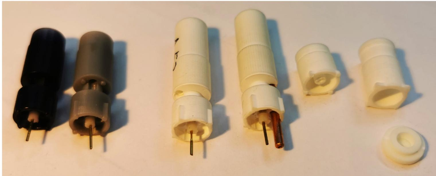
Two versions of end-plug have been developed for straw: standard and light (for the central hole).
