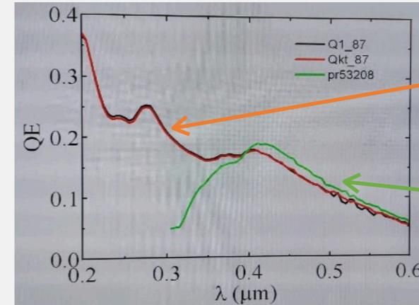
New Multi-Alkali PCs sputtered on quartz optimized to detect Cherenkov radiation
