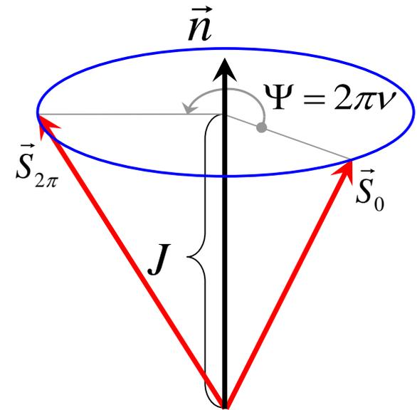
**In ideal accelerator**  $\vec{n} = \vec{e}_z$ ,  $\nu = \gamma G$   $G = (g - 2)/2$  – gyromagnetic anomaly
