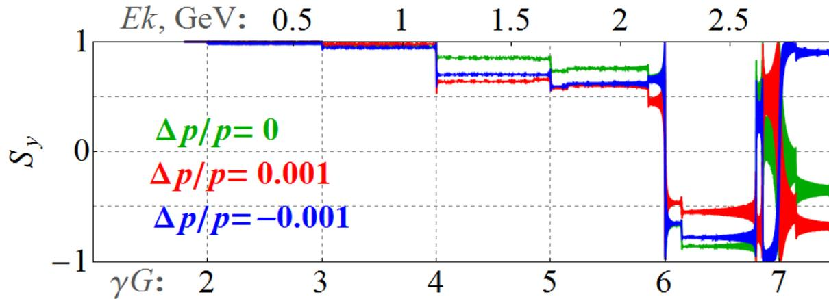
The vertical proton spin components during acceleration of three protons with different momenta in the Nuclotron without partial snake
