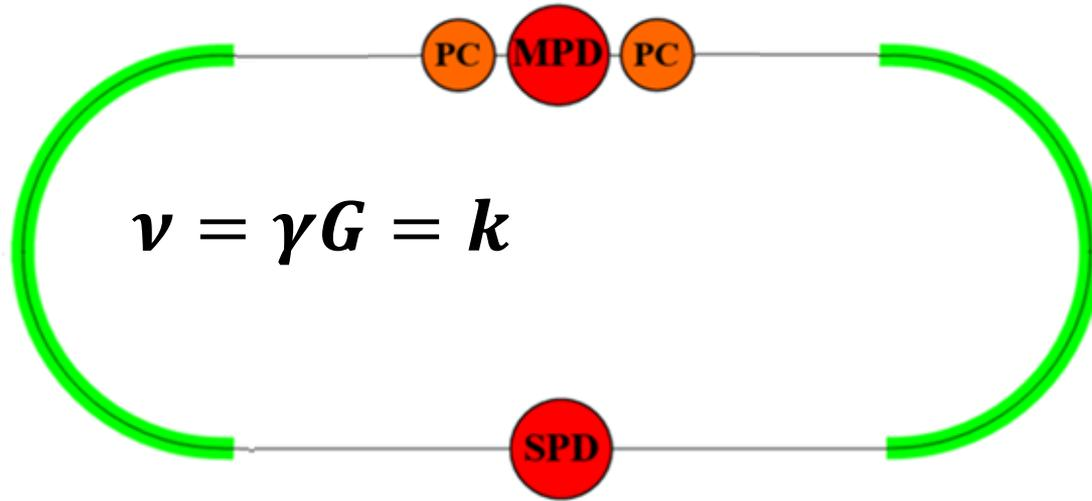
Spin transparency mode at zero-spin tune gives advantage even at energies which corresponds to the integer spin resonances  $\gamma G = k$ .
