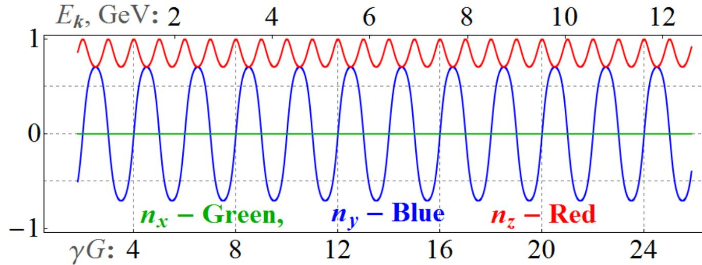
The  $\vec{n}$ -axis components at acceleration with the 50% solenoidal snake
