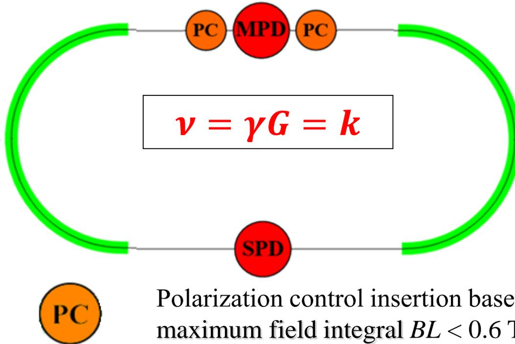
Polarized beam is injected from Nuclotron to the NICA collider at energy which correspond to integer spin resonance
