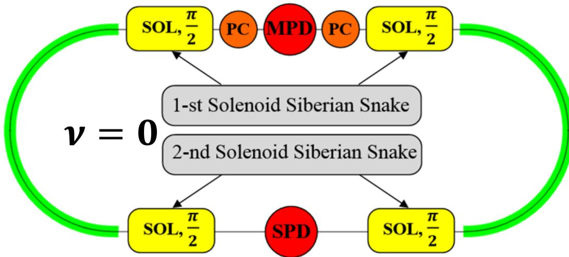
In the case of  $\nu = 0$  two **solenoidal snakes eliminate impact of synchrotron oscillations** on polarization which allow to significantly improve quality of polarized beam and increase lifetime of the polarization.
