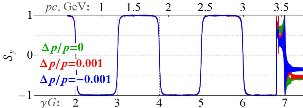
The 5% solenoid snake is required the solenoid field integral of **0.65 T·m** at the momentum of **3.4 GeV/c**.
