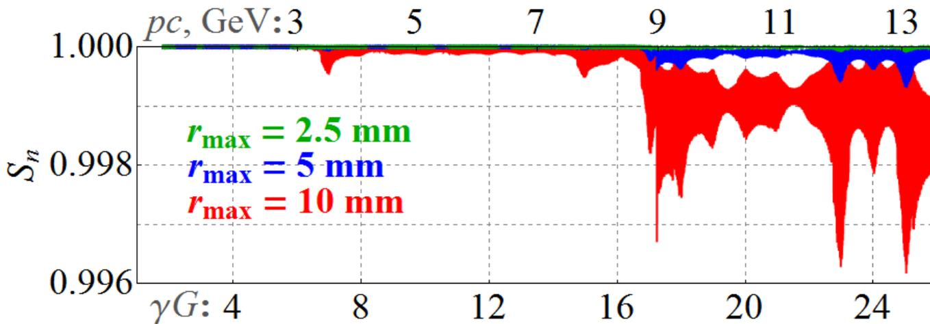
The  $S_n = \vec{S} \cdot \vec{n}$  projections at acceleration of three protons with the 50% solenoidal snake
