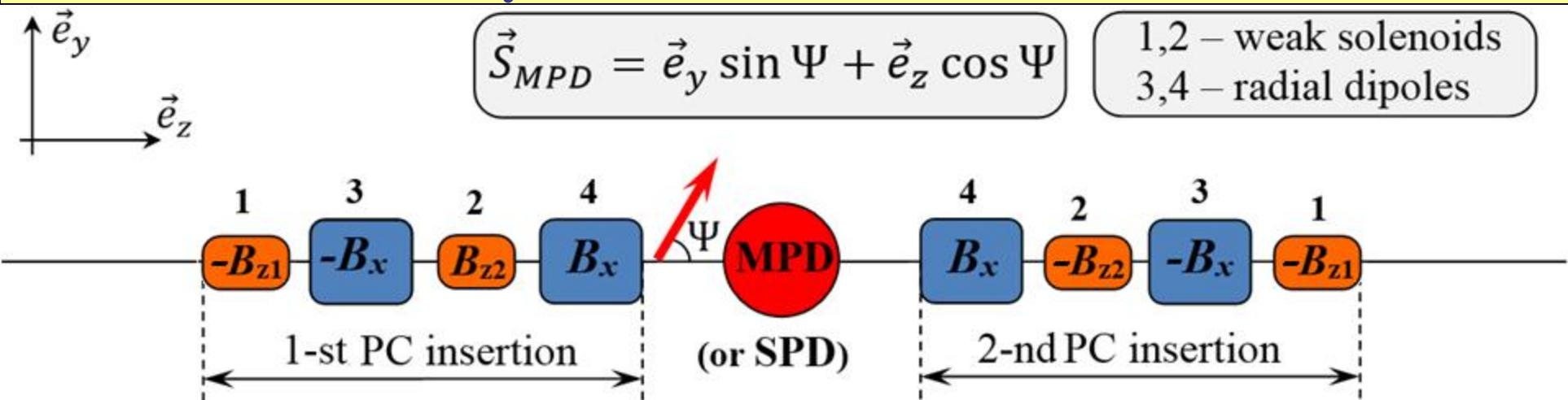
$\Psi$  is the angle between the polarization and velocity directions
