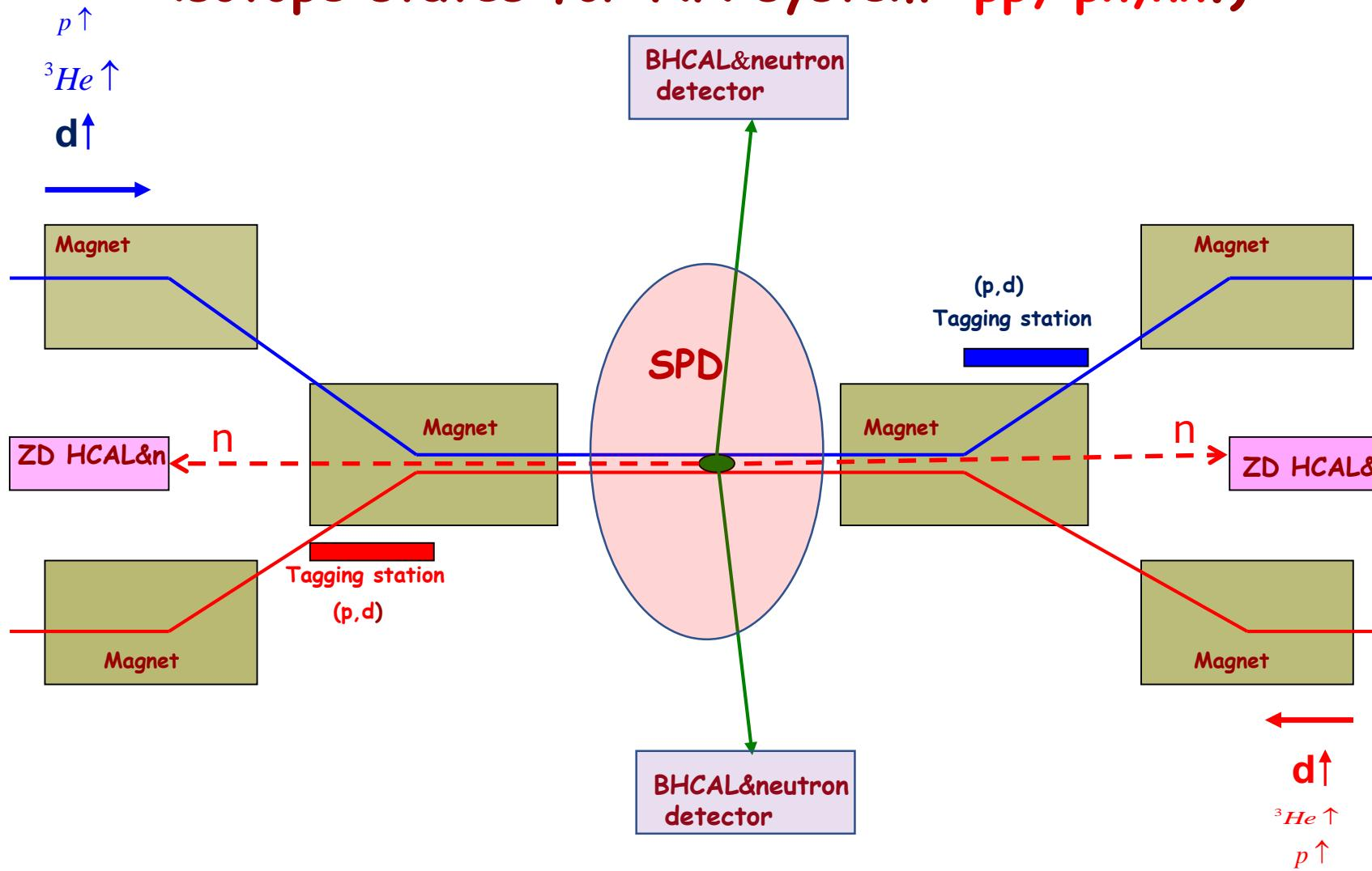
The tagging stations can be used as polarimeter!
