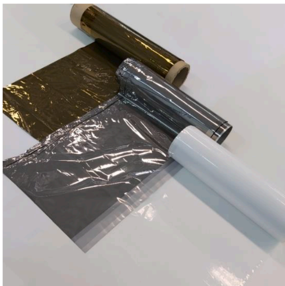
Fig. 2. Photo of TiO 2 -Ti-TM (goldish), Ti-TM (silverish) and TM (whitish) rolls.
