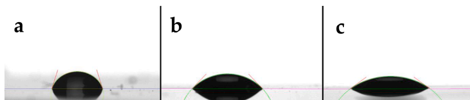
Fig. 13. Contact angle (a) TM, (b) Ti-TM, (c) TiO 2 -Ti-TM.
