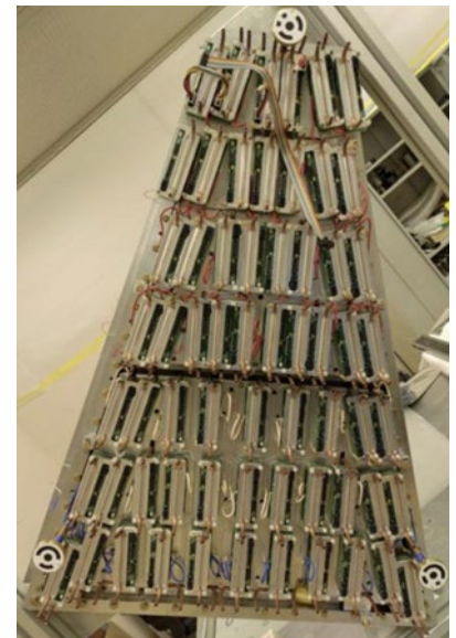
Fig.4 View of ROC chamber with installed readout electronics and cooling radiators.
