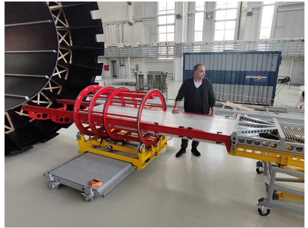
Fig. 8. Installation bench test
