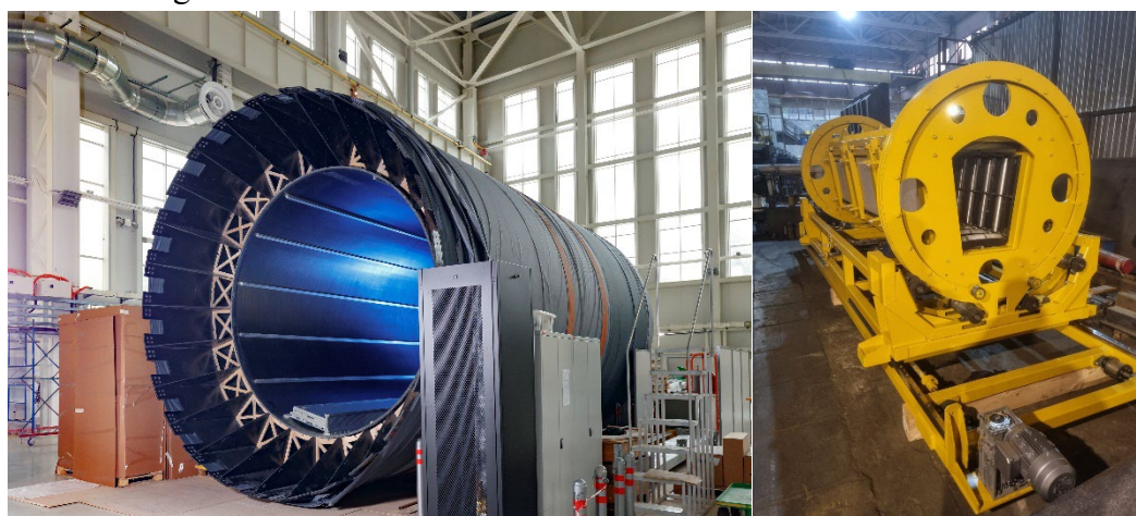
Fig. 3.7.9. Left panel: MPD power frame. Right panel: the tool for half-sectors installation.
