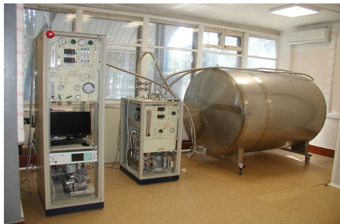
Fig.5 Testing of the gas system with the test volume in the LHEP bld.217.
