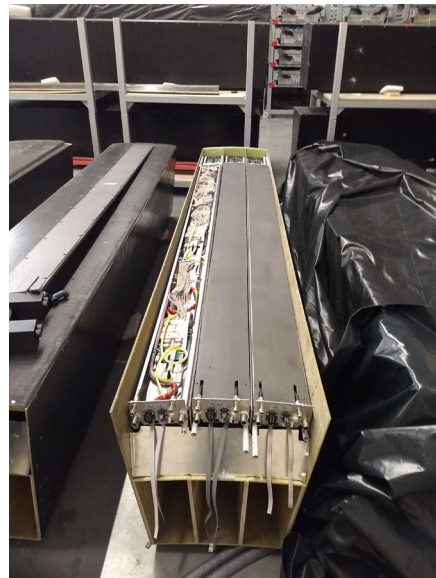
Fig. 3.7.6. Gluing of the clusters into the basket (left) and assembled half-sector (right).
