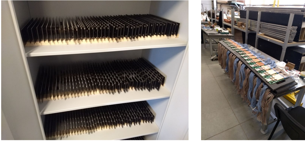
Fig. 3.7.2. Left panel: front-end boards. Right panel: ADC boards ready for installation.
