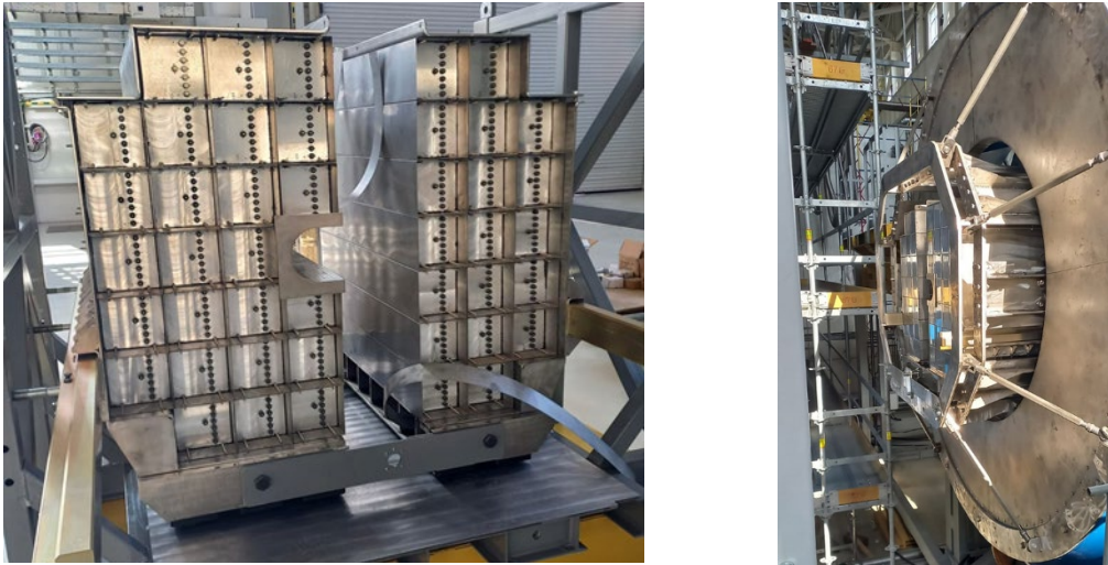
Fig.6 Left – Assembling of one FHCAL arm at floor. Right – FHCAL arm is installed in magnet pole.
