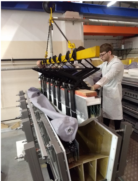
Fig. 3.7.6. Gluing of the clusters into the basket (left) and assembled half-sector (right).
