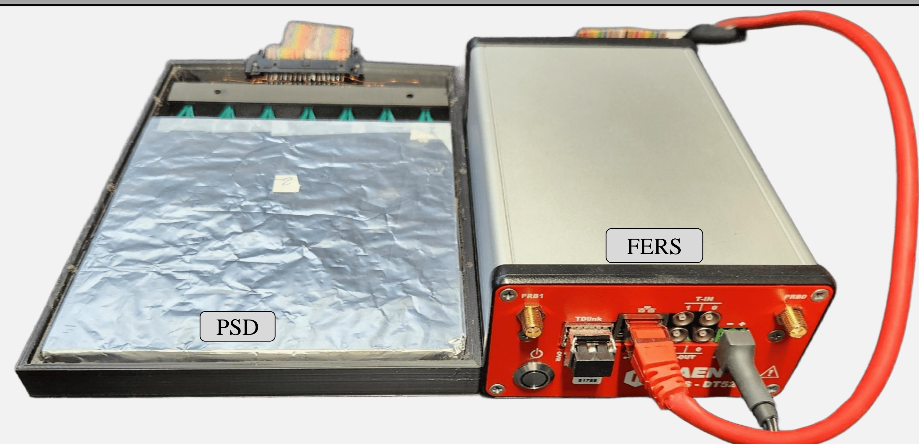
Fig. 2. The PSD next to the CAEN FERS DT5202 front-end electronics.
