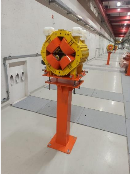
Quadrupoles installed and adjusted at beam line
