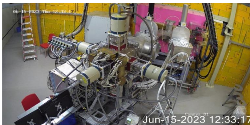
Fig. 1 GABRIELA-III detection system in the focal plane of the separator GRAND (left output). The right output in the focal plane, where the recoil nuclei collection chamber of the CryoDetector is located.
