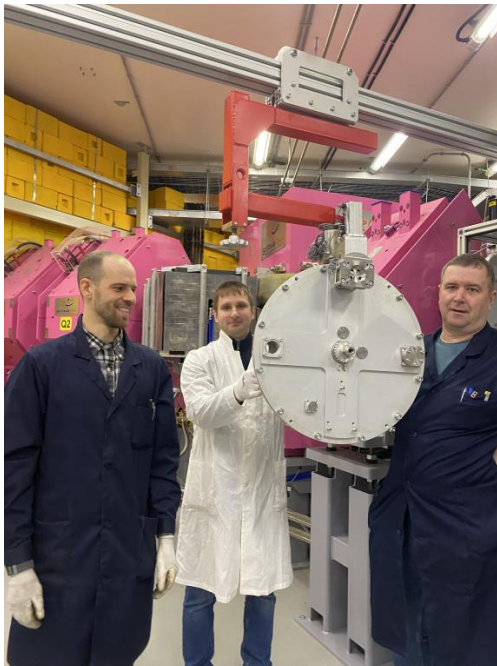
First tests of new rotating target D = 480 mm and 6 \mu\text{A} of ^{48}\text{Ca} SHE Factory, April 2024
