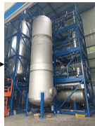
Distillation: remove radioactive impurities
