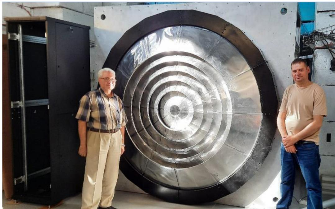
New large aperture ZnS scintillator detector system covering scattering angles range  $2\theta = 133-175^\circ$ , installed at the HRFD diffractometer.
