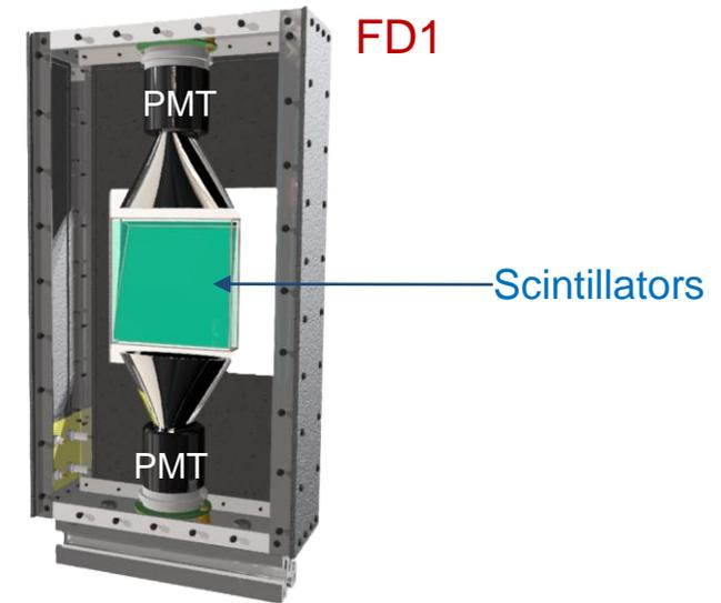
Measured with additional FD1 counter, placed behind the FHCAL hole.
