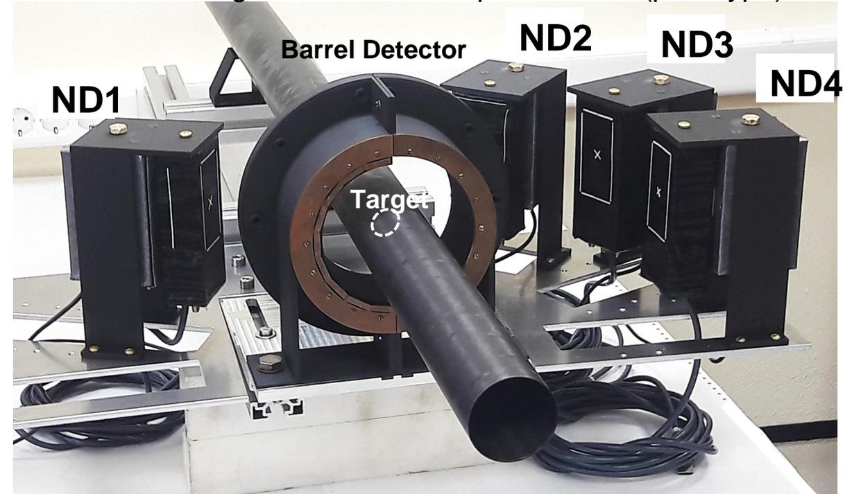
Compact time-of-flight spectrometer. Range of neutron energies from 1 to 200 MeV. With this spectrometer the neutron emission from target spectators in Xe + CsI collisions at 3.8 A GeV was studied by measuring double-differential neutron production cross section.
