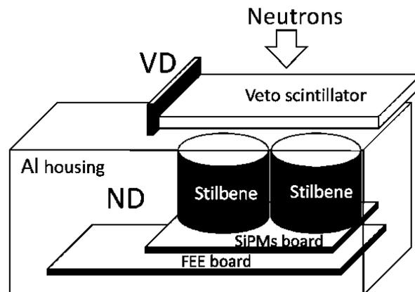
A new design of the neutron spectrometer (prototype)
