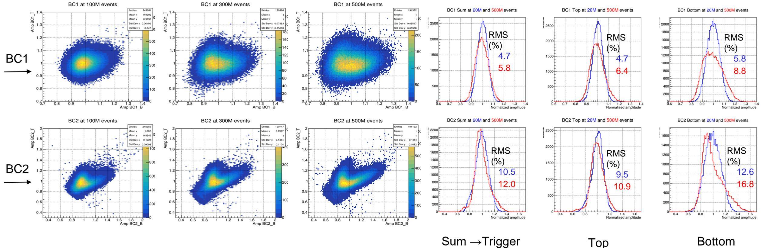
We see some degradation of the signals, which results in larger RMS at the end of the run – in BC1 Sum, BC2 Sum and individual signals.
