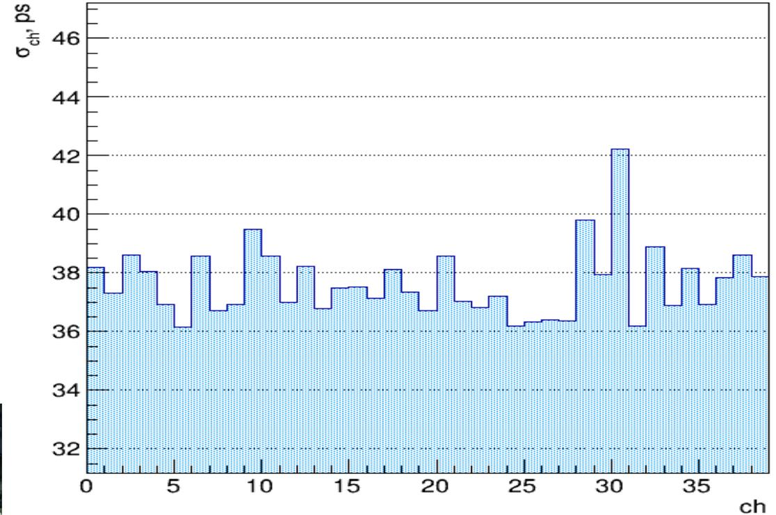
The TDC channel precision. Measured with the data generator DG2040 (Cycle-to-Cycle Jitter 5ps).
