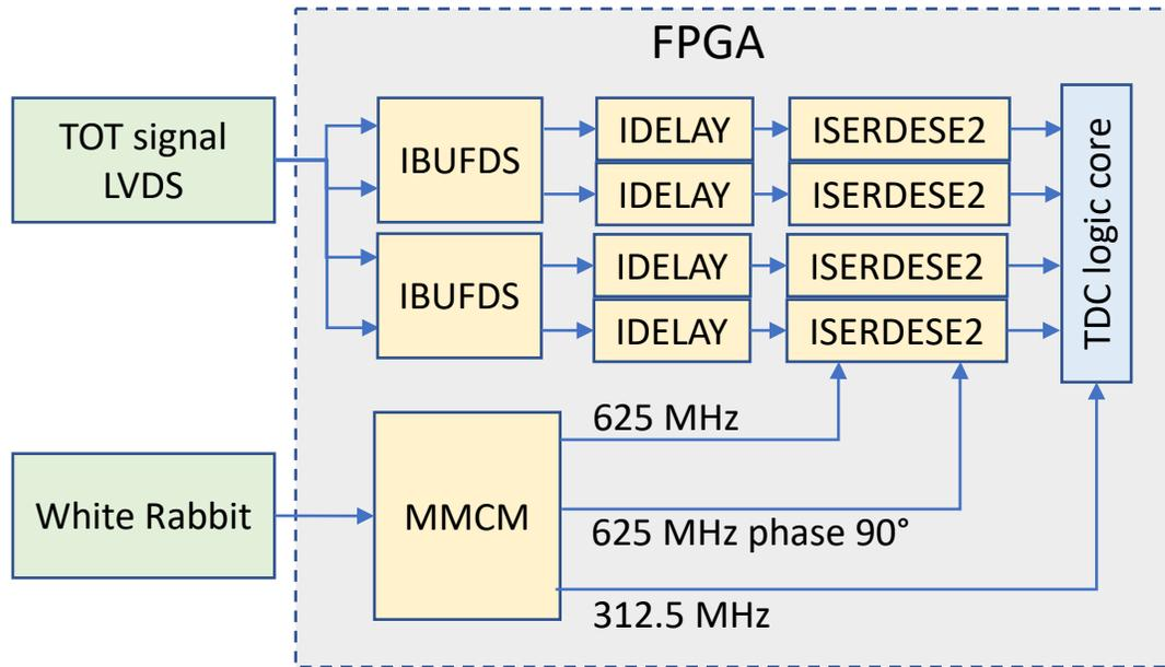
The TDC is **based on the Kintex-7** input serial-to-parallel converter with oversampling capability and programmable delay. The design is **based on Xilinx recommendations**, and uses **only documented features** of the FPGA within its specifications.
