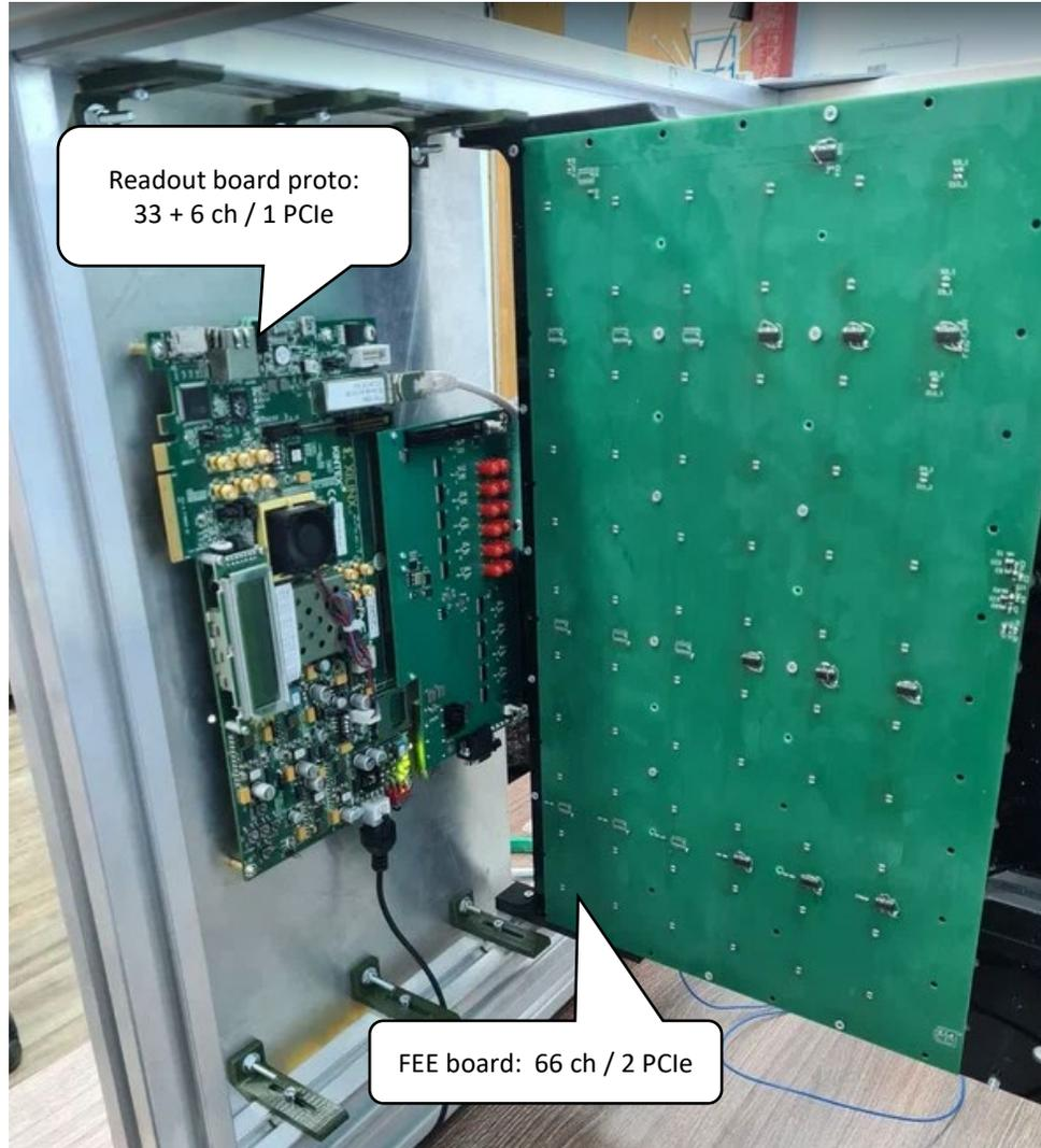
1/4 matrix readout prototype
