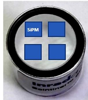
Detection of scintillation photons with four SiPMs 6×6 mm<sup>2</sup>, SensL, J ser.
