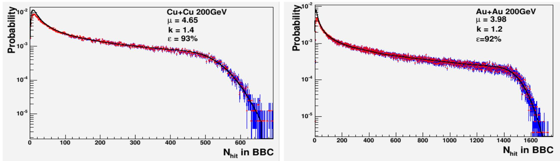
**Figure 3.** Distribution of the number of hits in both BBC (blue) fitted by the MCG-NBD function (red) for  $Cu + Cu$  and (left) and  $Au + Au$  (right).
