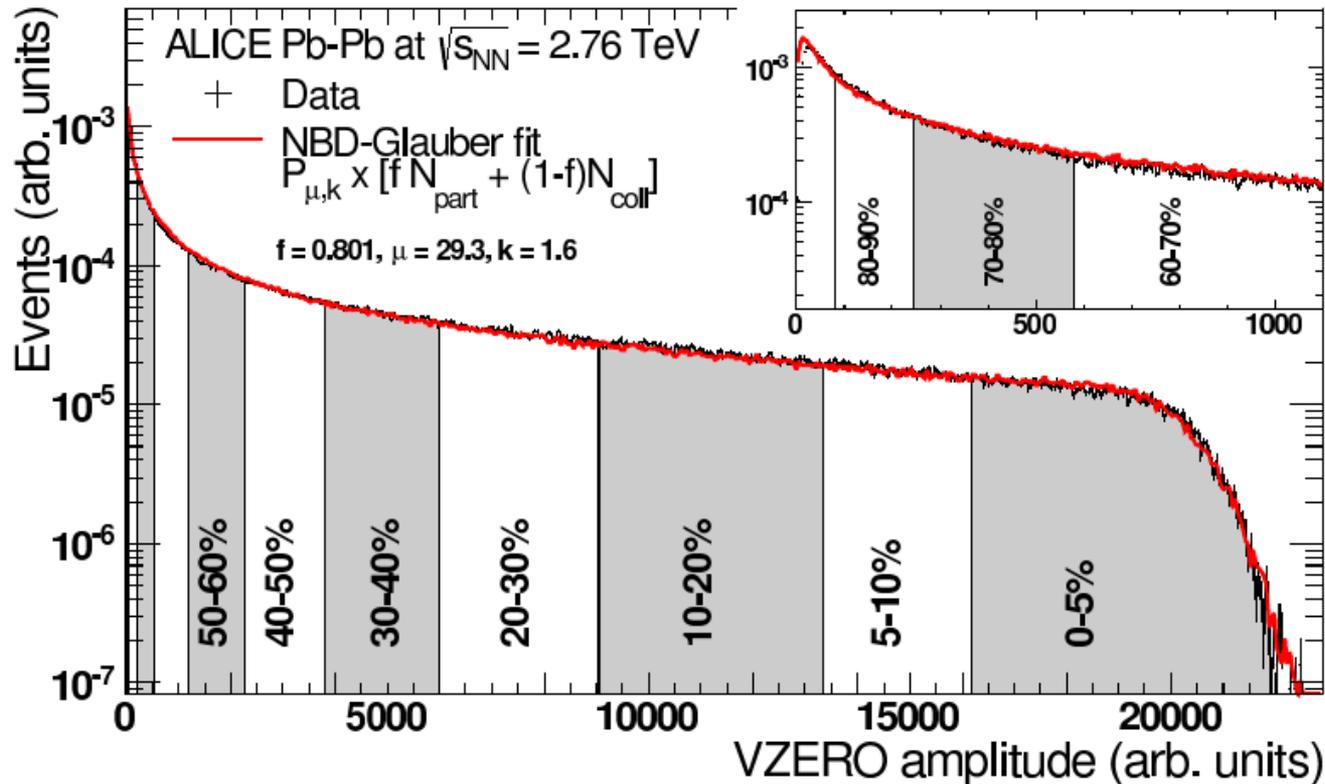
**Fig. 10:** (Color online) Distribution of the sum of amplitudes in the VZERO scintillators. The distribution is fitted with the NBD-Glauber fit (explained in the text) shown as a line. The centrality classes used in the analysis are indicated in the figure. The inset shows a zoom of the most peripheral region.
