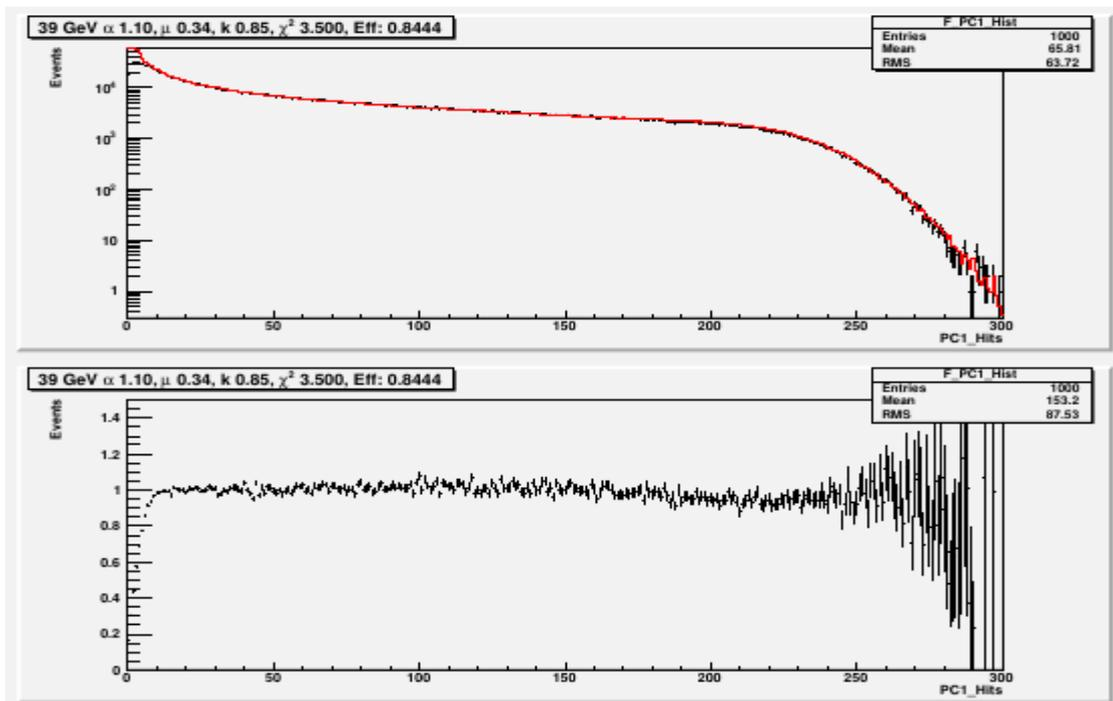
Figure 13: Upper panel: Example of NBD-fit of PC1 hit distribution for BBC-Z vertex cut  $|z| < 20$  cm and BBCLL1( $>1$  tubes). Lower panel: The resulting efficiency function plotted vs number of PC1 hits.
