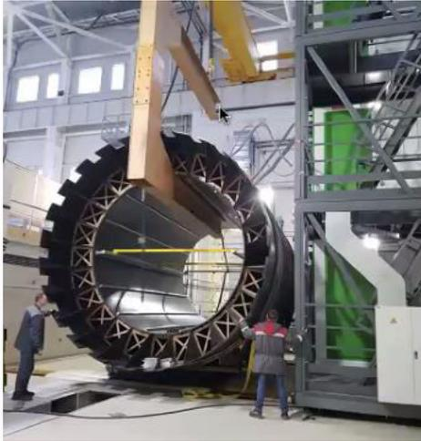
Carbon fiber support frame delivered and unpacked, sagita ~ 5 mm at full load, rails for the TPC and TOF are installed
