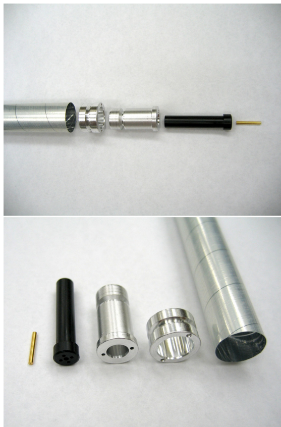
Fig. 7. Straw, donut, feedthrough, pinholder and crimp pin.
