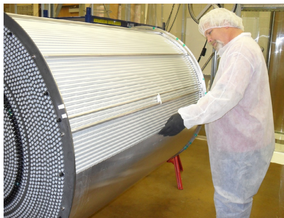
Fig. 6. Straw-tubes in layer 28, with one half of the outer shell in place.
