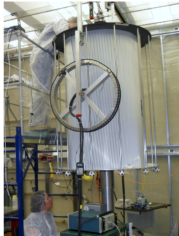
Fig. 8. Wire tension measurement being made. One Helmholtz coil is visible in the foreground.
