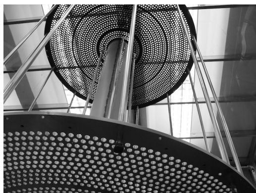
Fig. 2. CDC frame prior to the installation of the straw-tubes.
