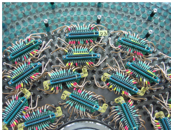
Fig. 11. Hookup wires and transition boards.
