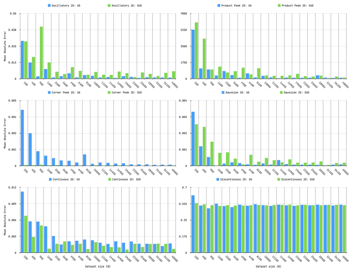
Figure 5: The Mean absolute error metrics relative to the type of dataset distribution ( UG - Uniform Grid and SUD - Standard Uniform Distribution) with different dataset sizes - [100, 40000]
