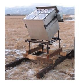
TAIGA-HiSCORE is a large-scale (1 km<sup>2</sup>) array of wide-angle non-imaging Cherenkov detectors, spaced ~100 m apart, designed to detect and study extensive air showers (EAS) from primary cosmic rays and gamma rays
