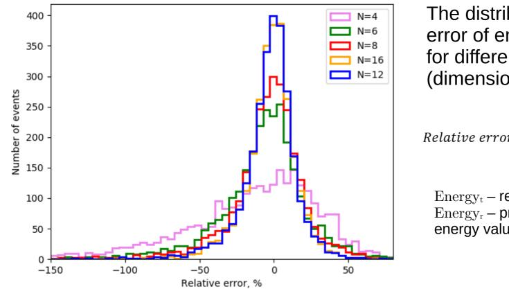
The distribution of the relative error of energy reconstruction for different values of N (dimension of the latent space):
