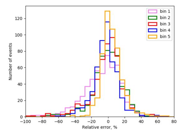
For N=12, we compare the distributions of relative errors of energy reconstruction for 5 different energy ranges (bins)
