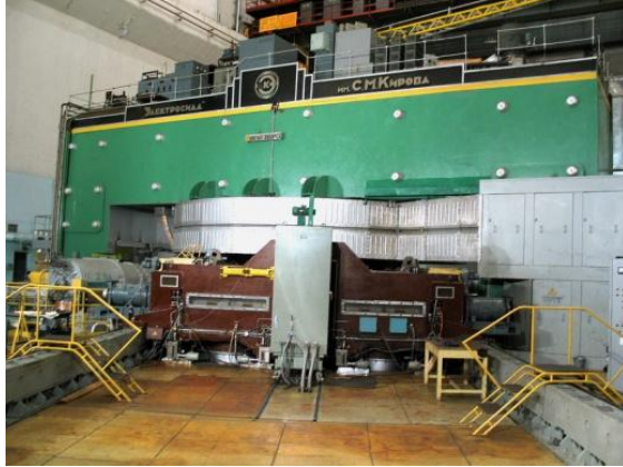
Phasotron: proton beam 640 MeV
