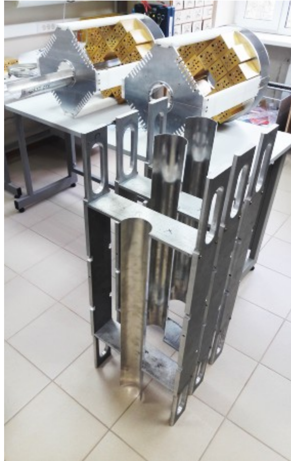
FFD mechanical support and tools for FFD installation
