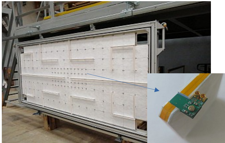
SiPM connector PCB on a tile
