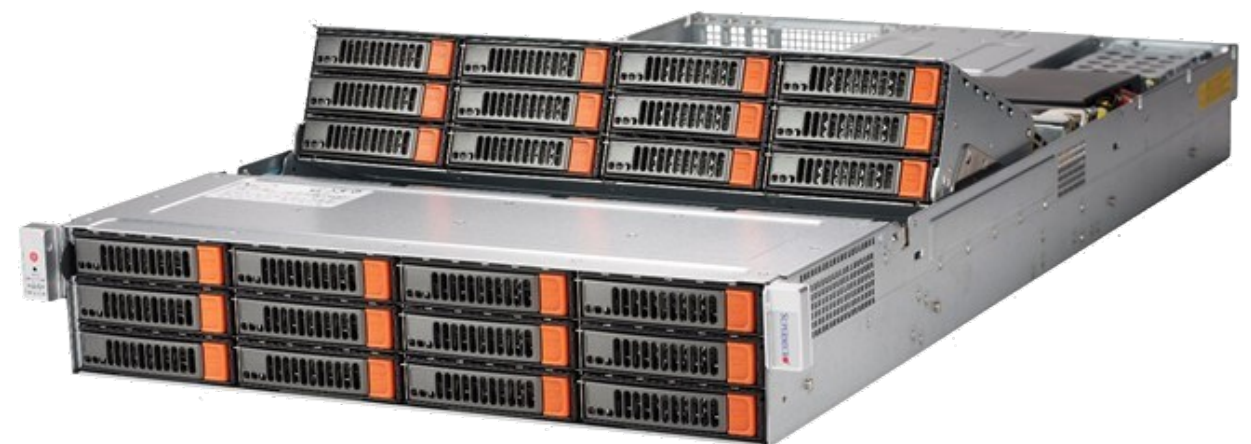
Ceph OSD node: 24 × 18 TB HDD
