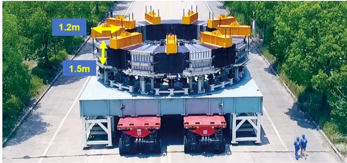
PF6 magnet, 12 m in diameter, ~400 tons
