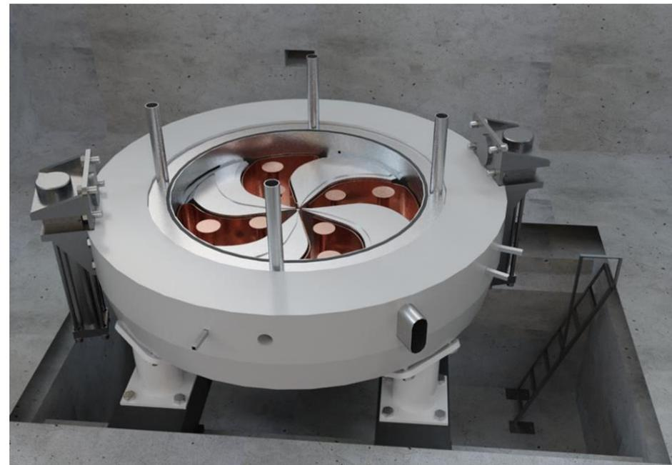
New superconducting medical proton cyclotron
