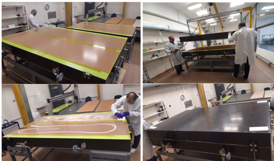
Fig. 10. Technological stages of the RPC panel production process
