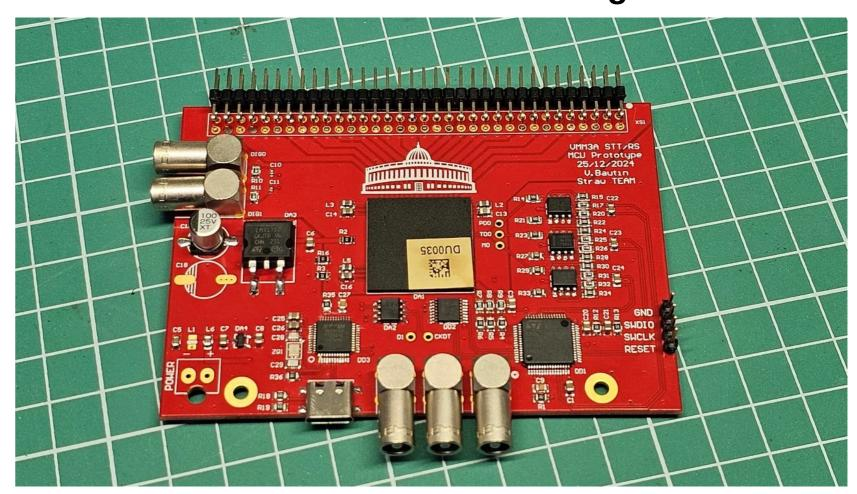
The new design utilize a non-commonly used mode of operation for the VMM3a ASIC. One can see significant improvement in the digitization resolution of the picture below. The main drawback is the speed. Operational hitrate has decreased to 10-20kHz per channel which is still feasible for the SPD Stage-I.
