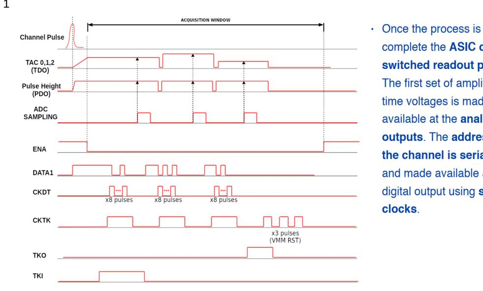
complete the ASIC can be switched readout phase. The first set of amplitude and time voltages is made available at the analog outputs. The address of the channel is serialised and made available at the digital output using six data
