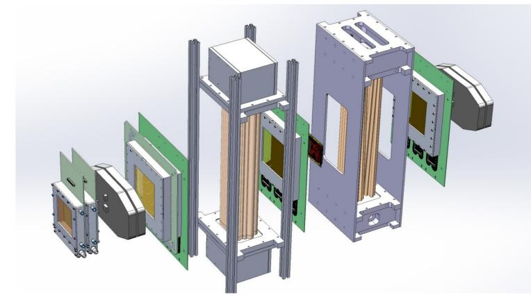
**StrawTrackerRD** setup at **CERN** (to be used in our nest FEE tests) T<sub>0</sub>: scintillator coincidence ~400 ps resolution. Reference tracking: micromegas + TIGER readout — track resolution: ~100 um
