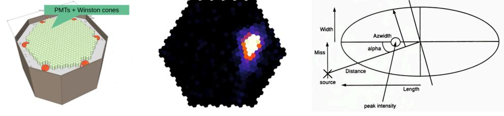
Fig. 2 Image of the Cherenkov camera with PMTs (a), example of an EAS event (b), Hillas parameters in the EAS image (c)
