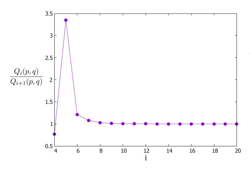
Convergence of the ratio of two subsequent iterations with an increase in the iteration number (i)
