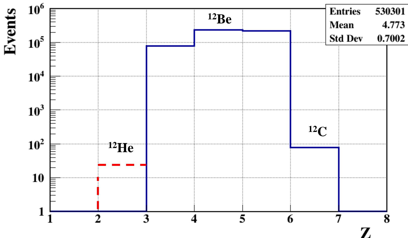
The output of fragments in the reaction  $^{12}\text{B} + ^{124}\text{Sn} \rightarrow \text{X}$  for A=12 and  $10^7$  interactions.
