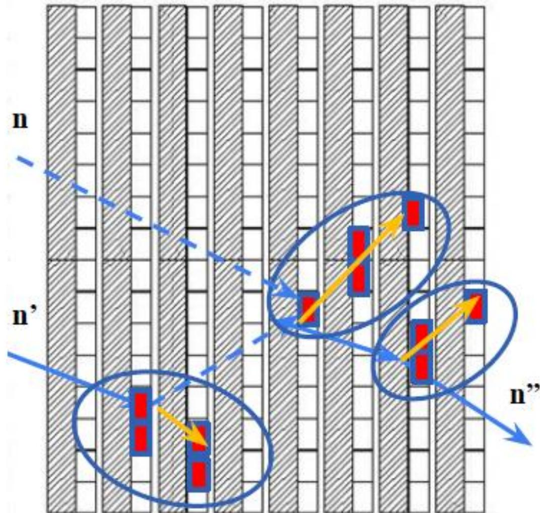
Registration of neutrons by a multilayer neutron detector. The layers are located at a distance sufficient to eliminate the interacting neutrons from the analysis.
