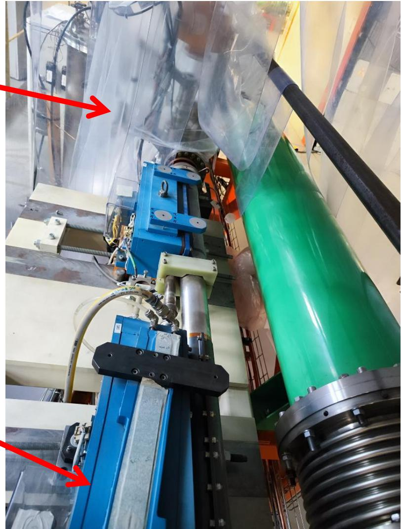
Mounted foils on the comb of the stripping station.
