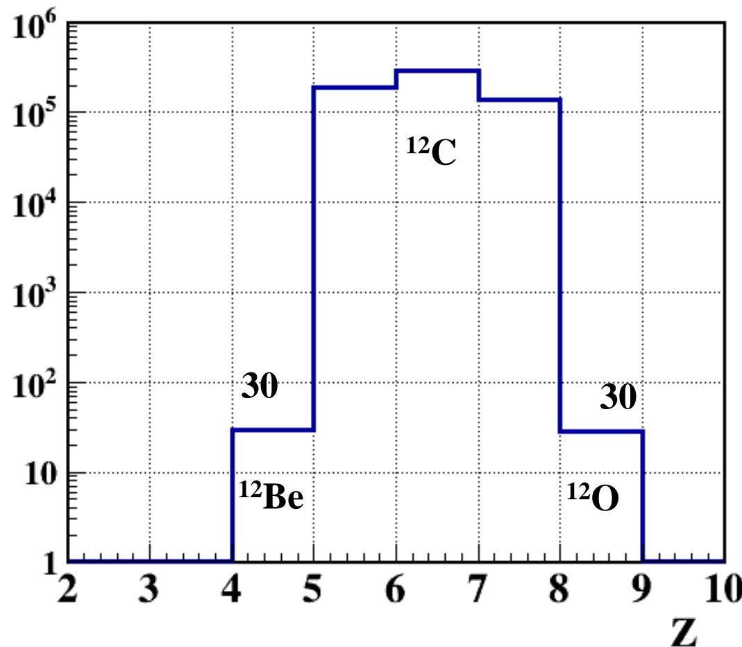
**Separation of fragments in the reaction  $^{12}\text{C} + ^{124}\text{Sn} \rightarrow \text{X}$**
