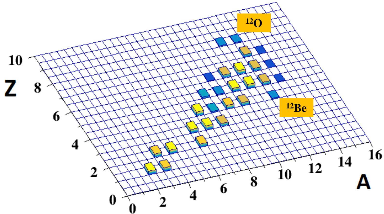
The yield of fragments in the reaction  $^{12}\text{C} + ^{124}\text{Sn} \rightarrow \text{X}$  for A=12 and  $10^7$  interactions.
