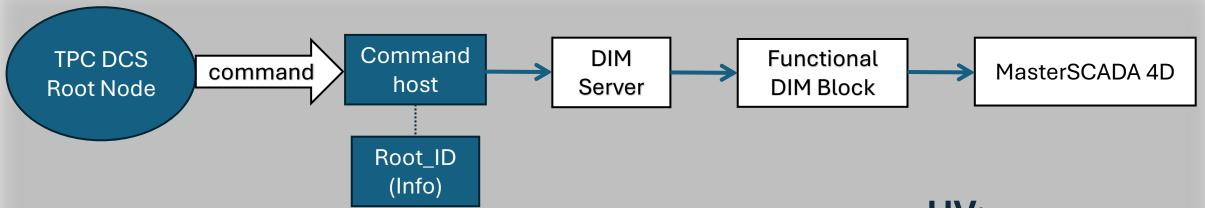
When external management is enabled, commands change the state of the corresponding SCADA variables.
