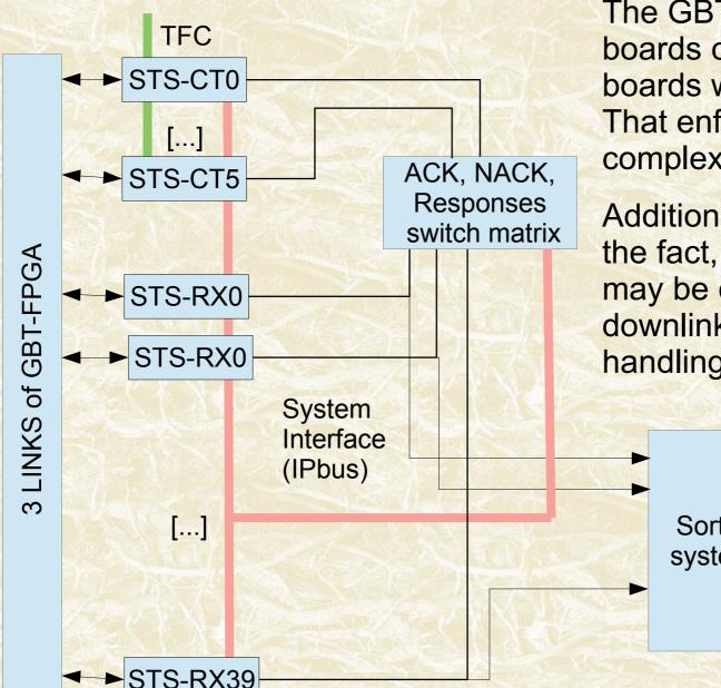
The GBT-based readout uses CROB boards connected to multiple FEB boards with multiple STS-XYTERs. That enforced creation of multilevel complex hierarchy of cores.
