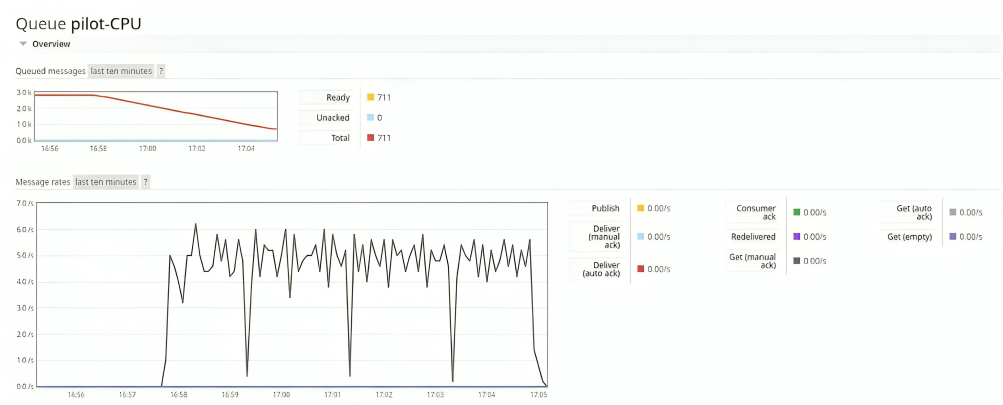
Рис. 6: 100 concurrent Pilots processed \approx 2,100 jobs in 7 minutes ( \approx 15 s/job including stage-in/out) on standard JINR Cloud VMs using a simplified synthetic payload.
