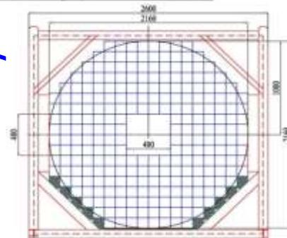
2x2 m<sup>2</sup> electromagnetic calorimeter, ECAL0<sup>3</sup>
